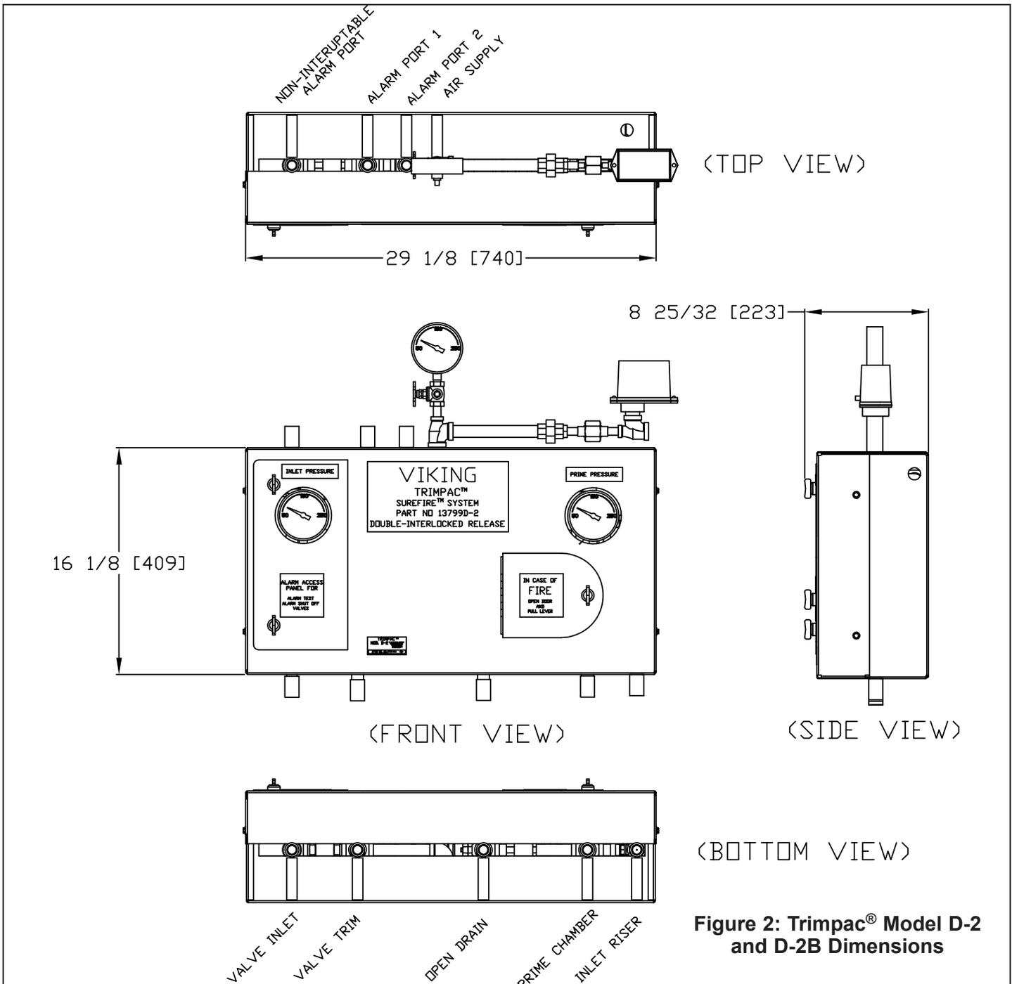
**Figure 2: Trimpac® Model D-2 and D-2B Dimensions**
