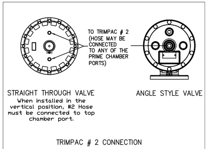
**Figure 11: Valve Connections**
